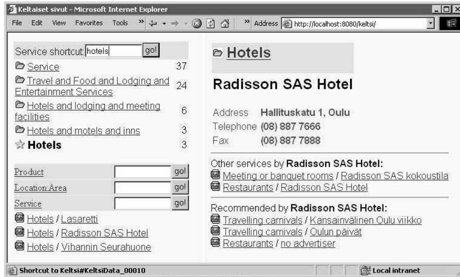
Fig. 2. The user interface is divided into two parts: on the left hand side is the ontology-based searching tool and on the right is the semantic instance browser.
